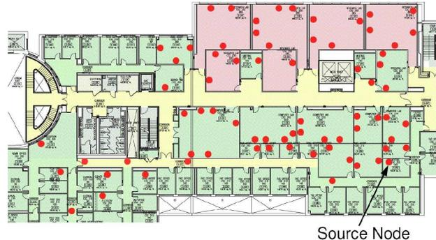
Fig. 7. The WiSeNet testbed (72 MicaZ motes; 152.5 feet  $\times$  97 feet).
